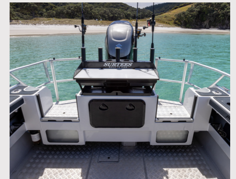
Offshore Transom with double walk through and two live bait tanks
