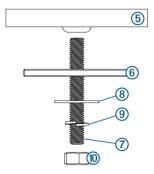
**9** Using a torque wrench, tighten the nuts to 13.7 to 18.6 N-m (10 to 14 lbf-ft.).
