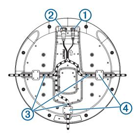
3 Press the cables into any of the guide grooves ③ on the bottom of the case, and secure them using a cable holddown plate ④.
