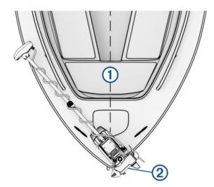
• You must install the mount with the u shape ② overhanging the gunwale of the boat.
