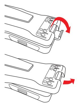
To re-fit the battery pack, slide the top of the battery pack in towards the radio then press the base of the battery pack downwards against the battery contacts. Rotate the battery lever upwards and press into place so that it clicks firmly.
