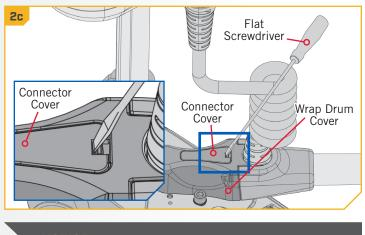
**NOTICE:** Please note the orientation and routing of the plug and wires for re-installation.
