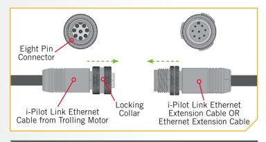
**NOTICE:** The connectors are keyed to prevent reversed installation.
