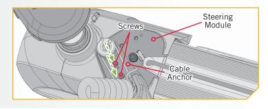
Using a #3 Phillips screwdriver, tighten the Cable 0. Tension Screw located at the base of the Toe End of the Foot Pedal to 10 - 12 in-lbs until the Steering Cables are under tension or re-tighten the same number of turns as was used in step 4f.
