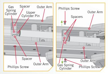
**NOTICE:** Use a #3 Philips screwdriver to remove the screws. They have a pre-applied thread locker. Not using the recommended tool can cause damage and prevent them from being removed.
