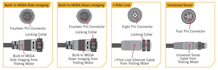
If **one** connection below the Control Head is present, the motor may be equipped with:
