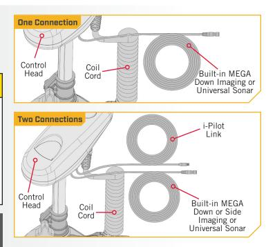
c. The cable(s) should be fed all the way through the Coil Cord. It/they should exit the Coil Cord at the bottom
