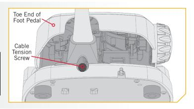
Reconfirm that the Steering Cables are tight and k. then carefully thread the Steering Motor Connection Wire through the top of the Wrap Drum Cover. The male plug comes from the Cable Anchor through the opening at the bottom of the Wrap Drum Cover. The wire with the female plug that runs out the top of the Cable Gear should also be pulled through the opening at the bottom of the Wrap Drum Cover.
