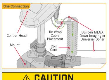
Do not over tighten the cable ties as it may damage the wires.
