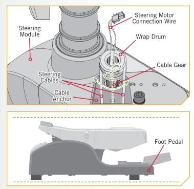
n. Re-tighten the two screws that fasten the Cable Anchor to the top of the Steering Module using a #2 Phillips screwdriver. Tighten to 25 in-lbs.
