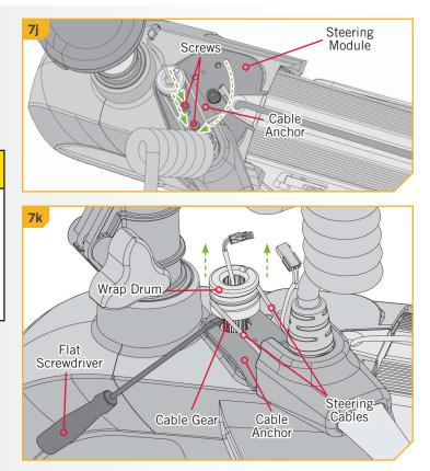
While holding the Wrap Drum just above the Cable Gear, and maintaining tension on the Steering Cables, carefully rotate the Wrap Drum right or left until the top of the Foot Pedal is parallel with the deck of the boat. The proper position of the Wrap Drum will locate the anchors for each of the Steering Cables equidistant from the mid-line of the Cable Anchor where it is secured to the Steering Module.
