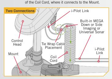
Use a tie wrap cable to secure the cables to the top d. of the Coil Cord, leaving only enough slack to let the cables hang comfortably.
