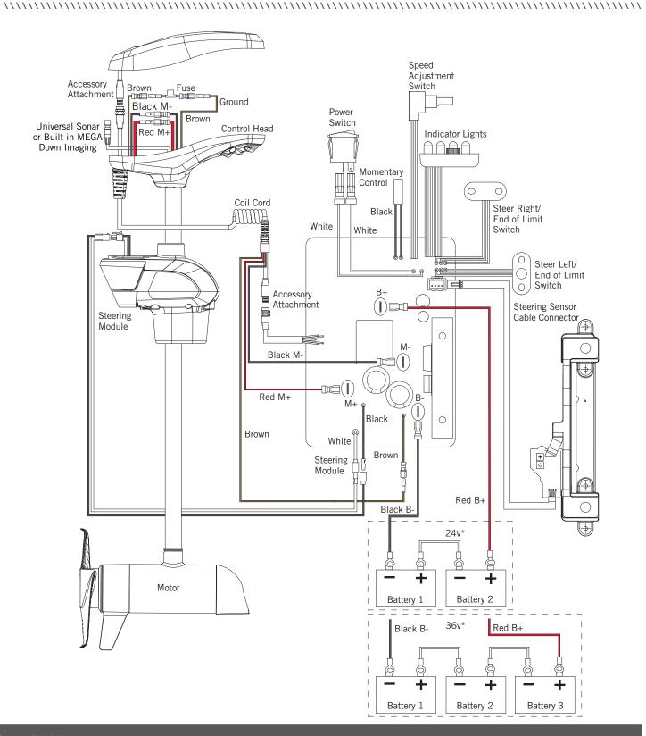
**NOTICE:** This is a multi-voltage diagram. Double-check your motor's voltage for proper connections. Over-Current Protection Devices are not shown in this illustration.
