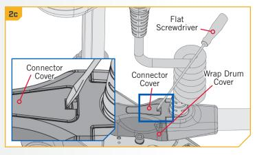
**NOTICE:** Please note the orientation and routing of the plug and wires for re-installation.
