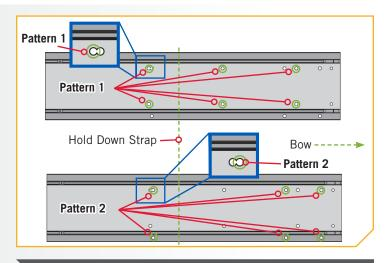
**NOTICE:** If Pattern 2 is used, the right side plate must be removed to access the mounting holes in the base of the Mount.
