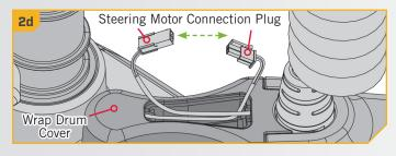
e. Remove the two screws that hold the Wrap Drum Cover in place with a #1 Phillips Screwdriver. Once removed, lift the Wrap Drum Cover away from the Steering Module.
