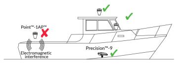
Point™-1AP™ and Precision™-9 compasses contain a magnetic heading sensor and should be mounted away from magnetic interference. The sensor should be mounted as level as possible in a location close to the vessel's center of pitch and roll.
