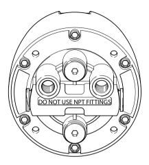
Text engraved on the back of this SeaStar® helm pump helps you identify the correct fittings.
