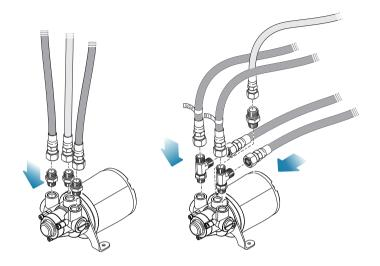
→ Note: You can connect tee connectors to the pump if space is limited behind the helm.
