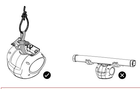
\Lambda Warning: Do not lift the pedestal with the antenna attached.
