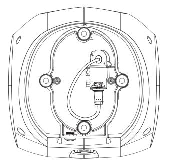
**Warning:** You must perform the following instructions BEFORE connecting the interconnection cable to the pedestal. Any adjustment to the cable length, angle and twist must be made before plugging in the cable.
