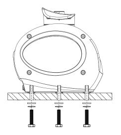
If you're installing the pedestal onto a steel surface, also use the supplied plastic isolating washers.
