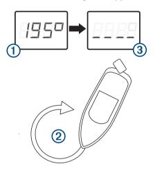
6 Within three minutes, complete two full, slow, tight circles ②, taking care to keep the boat as steady and level as possible.
