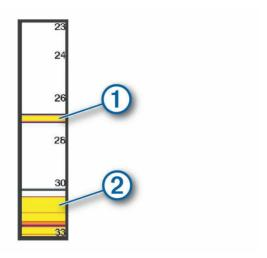
The a-scope above shows fish returns  $\bigcirc$  and a soft bottom return  $\bigcirc$ .
