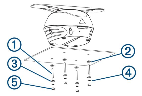
To avoid damaging the pedestal, you should stop tightening the threaded rods when they no longer turn easily.
