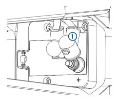
2 If necessary, clean any corrosion from the terminals using a wire brush.
