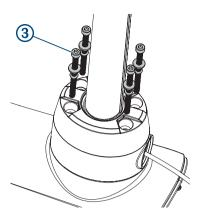
When replacing the transducer, you should dispose of these four screws. New screws, washers, and O-rings are provided in the shaft and motor hardware service kit.
