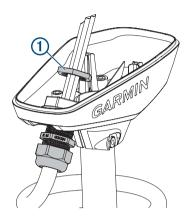
2 Pull the coil cable out of the shaft cap to remove it.
