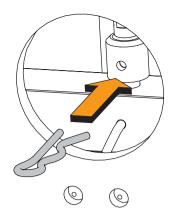
3 Feed the other end of the pull cable through the steering servo housing, routing the cable between the upper link of the mount and the pivot pin.
