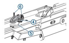
7 Using a #2 Phillips screwdriver, install the two screws (6) that secure the lower gas spring clevis to the lower link of the mount.
