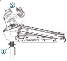
2 Slide the shaft down and out of the steering servo, taking care not to damage the skeg and transducer or snag the cables or connectors ② as you pull it through.
