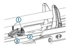
3 Lift the lower gas spring clevis off of the safety rod 3.
