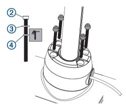
14 Using the grease packet included in the shaft and motor hardware service kit, apply grease to the 4.75 mm (<sup>3</sup>/<sub>16</sub> in.) O-ring on each bolt.
