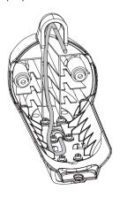
**11** Place the nose cone onto the propeller drive motor.
