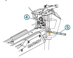
5 While lifting up on the steering servo housing, push the pivot pin (5) through the housing and the link to hold it in place.
