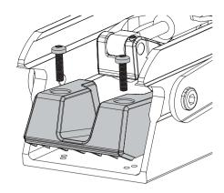
2 Install the replacement stow support using the screws provided with the replacement part.
