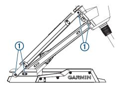
**2** Apply a non-stick, dry-film lubricant to each hinge point, in the space between the moving parts ②, and allow it to dry according to the instructions provided with the product.
