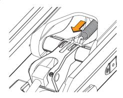
**9** Install the steering servo on the mount (*Connecting the Steering Servo to the Mount*, page 20).
