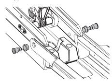
**TIP:** The bolts that secure the upper link to the mount base are fastened very securely at the factory. You may need to
