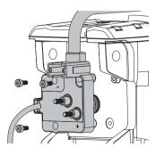
4 Using a 4 mm hex bit or screwdriver, insert and tighten the three screws to secure the coil cable block to the steering servo housing.
