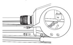
4 Remove the pull cable from the mount base, and pull it through the steering servo housing.
