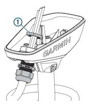
3 Using a 36 mm or adjustable wrench, tighten the plastic nut on the coil-cable connector inside the shaft cap
