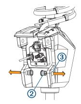
4 Holding the pull cable 4 up, place the steering servo housing onto the lower link of the mount, aligning the lower holes on the housing with the holes on the link.
