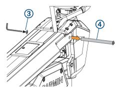
**TIP:** It is helpful to use another 4 mm hex wrench to hold one end of the upper pin stationary while you remove one screw.
