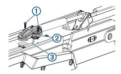
2 Lift the upper gas spring clevis off of the safety rod 3.
