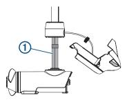
**12** Gently pull the ends of the power and data cables as you feed them the rest of the way through the shaft.
