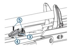
7 Using a #2 Phillips screwdriver, install the screws<sup>5</sup> that secure the lower gas spring clevis to the lower link of the mount.
