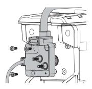
2 Pull the coil cable block away from the steering servo housing to remove it.
