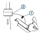
3 After you have fed all but approximately 60 cm (2 ft.) of the transducer cable through the hole in the shaft base, feed the transducer cable up through the shaft.
