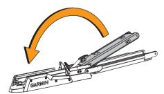
2 Push the two safety rods ① into the lower link as far as possible.
