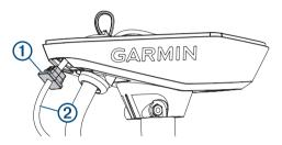
6 Remove the grommet from the transducer cable.
