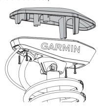
You should place these screws in a safe place, because you must use them to close the shaft cap.
