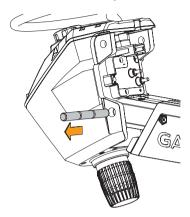
The steering servo is no longer connected to the mount.
