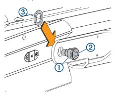
2 Place a plastic washer ③ that you removed with the original upper link or a washer supplied with the replacement upper link between the upper link and the mount base.
