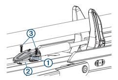
**NOTE:** If you must rotate the gas spring so the base aligns with the mount, rotate the spring in a clockwise direction only. Rotating the gas spring in a counter-clockwise direction may loosen the fittings.
