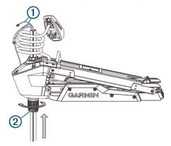
**TIP:** Depending on the height of your trailer or workbench, you may want to move the motor mount up about halfway to make it easier to install the shaft.
