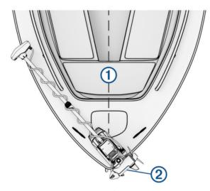
• You must install the mount with the top of the cutout ② overhanging the gunwale of the boat. The U shape should extend over the side of the boat.
