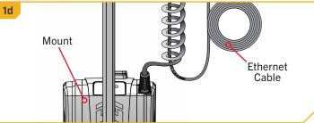
**NOTICE:** Minn Kota recommends routing the Ethernet Cable through the Coil Cord. Bypassing the Coil Cord when routing the Ethernet Cable is not recommended.
