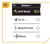
**NOTICE:** For quick customization, press and hold the OBN button you want to customize to quickly bring up the customization screen.
